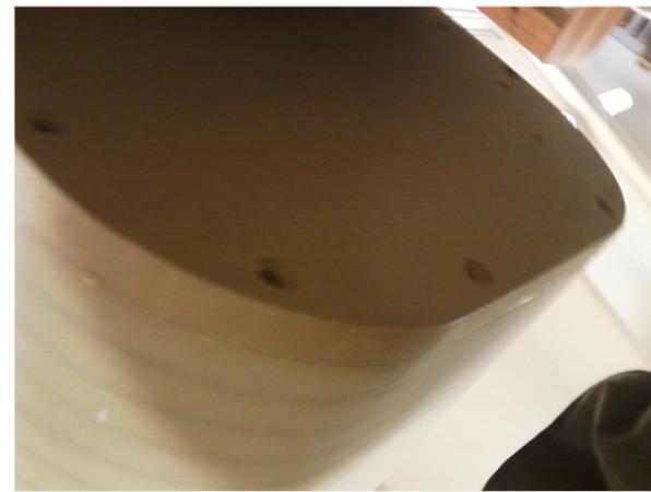
This is how the back was connected. It was screwed in place ever 100mm. The places where the screws would be screwed in place were first pilot holed and the counter sunk to make sure that when it was connected to the wall it would sit flush against it. It would also have no sharp edges when it is being carried around etc. Once the glue had dried the edge was sanded flat and all of the sharp edges were removed
