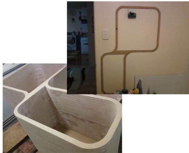
This photo shows what the unit looked like when it was ready to be painted. The first thing that need to happen before this was to get the back connect (glued and screwed) By being proactive I had brought the back home already to work out where the holes would go so that it would be strong against the wall.
