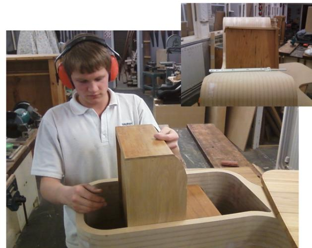
Here you can see that I have fitted the old drawers using the big belt sander so that once I have the unit back from being painted all that I will need to do is fit the drawer runners
