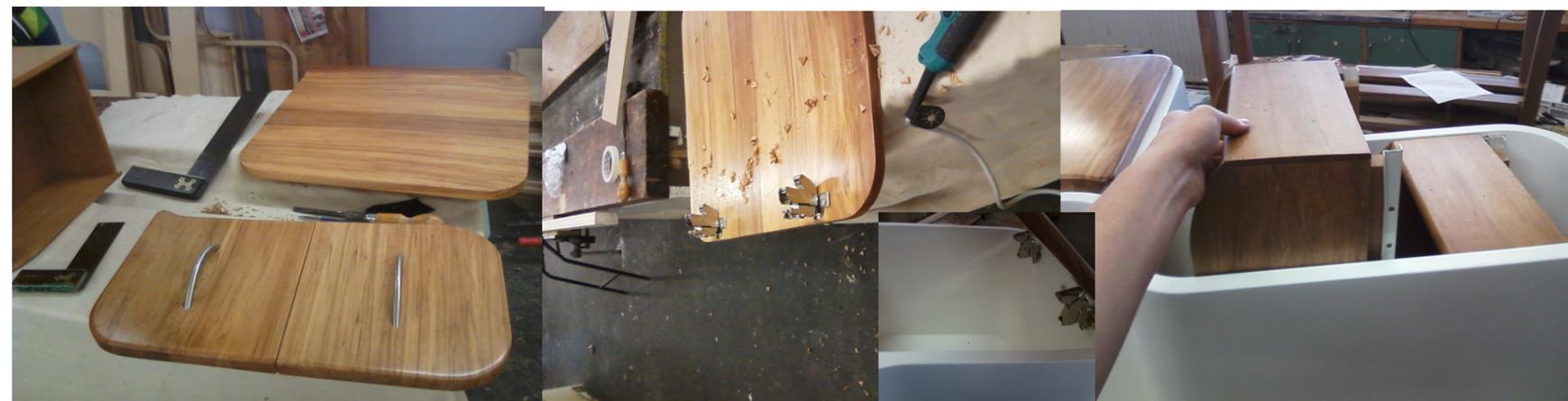
Here you can see that I am adding some of the finishing touches to the doors and drawer fronts by putting on the handles. This is another thing that I did to save time as now once the drawers have been fitted I just need to screw the fronts in place.
