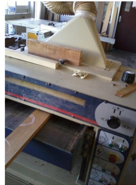
While I waited for the unit to be painted I got the wood that I would be using for the drawer fronts door and shelf ready. The first thing that I needed to do was get them all down to the right thickness using the thicknesser. When I was using this machine I made sure I had covered shoes and ear muffs to protect my feet and ears.
