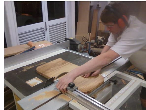
Now I am cutting the drawer fronts into the 2 separate drawer fronts using the table saw. When I was using the table saw I made sure that my hands were away from the blade and I held the piece that I was cutting securely. I also was wearing covered shoes glasses and earmuffs to protect my feet eyes and ears.
