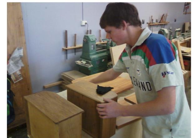
Here I am varnishing the door, drawers, drawer fronts and shelf. This will make them moisture and heat resistant while also being hardwearing. 3 coats were applied with a quick sand with white sand paper in between each coat.
