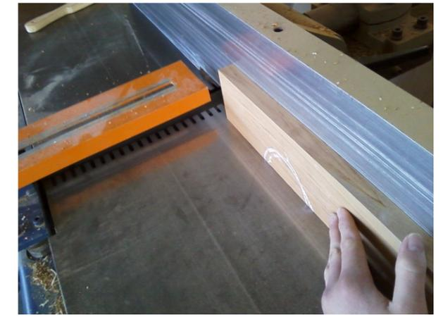
Next the edges needed to be surfaced so that the different pieces could be glued together with no gaps. This was done to all the different pieces. Then the wood for the shelf door and drawer front were glued together and left the dry in a in the clamps.
